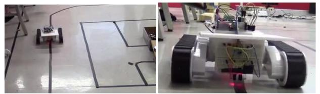
Figure 3: Line Tracing with Two LEDs and Light Sensors
