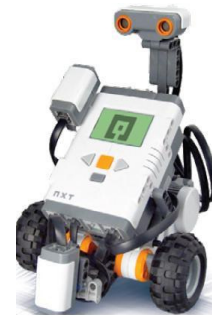
Fig. 1. Basic setup of the LEGO MINDSTORMS NXT robot used in most of the camp activities
