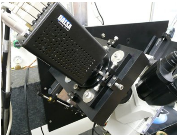
Figure 5. KESM camera and objective focusing controls.
