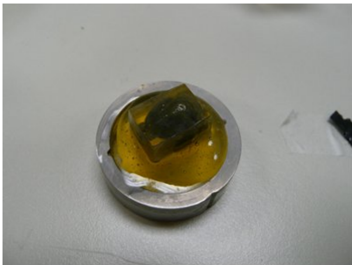
Figure 2. Embedded mouse brain specimen mounted on the specimen ring.
