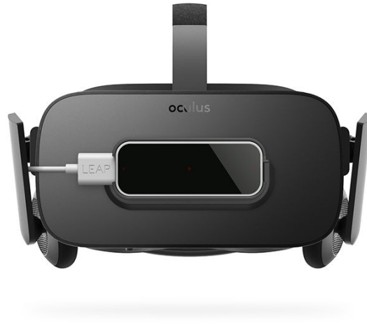
Figure 8.10: Leap Motion Controller mounting on the Oculus Rift [37].
