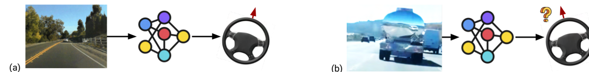
Figure 4. ML model problem due to simple association of input with output. (a) An ML model trained with pairs of images from a front-facing camera and steering angle. The ML model works well as long as the input has a similar distribution to training datasets. (b) Even a successful model will show unexpected behaviors when the input data has a significant distributional shift (a reflected road image on the car in front) from the training datasets.
