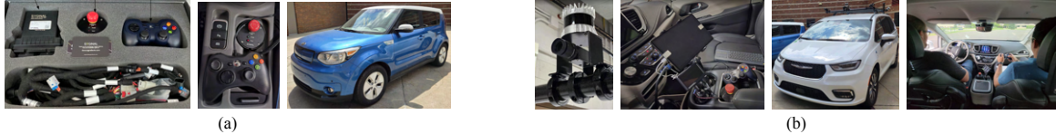
Fig. 11: (a) Kia Soul EV with a Sygnal DBW system and (b) Chrysler Pacifica Hybrid with a sensor suite. The DBW kit includes brake, throttle, steer, and shift-by-wire controller modules. It also has the following features for research and development for autonomous driving: driver override by pressing the brake, throttle, shifting, or turning the steering wheel. The sensor suite includes the following components: one high-resolution 64-channel LIDAR, two 32-channel LIDAR, four RGB cameras, and one GPS antenna
