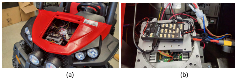
Fig. 4: Power and Wiring. Without re-wiring, the proposed DBW module can reside under the vehicle's hood. (a) The hood is open. Everything will be under the hood. (b) The onboard controller is in action.
